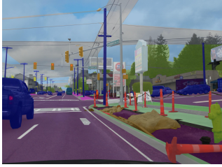
Figure 5: An example of semantic segmentation overlaying with the original image from the Mapillary Vistas Dataset.
